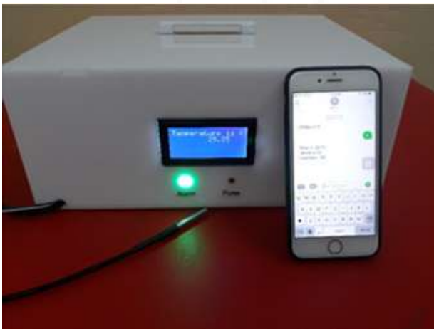
Figure 4: sending a message, the device sends "Problem" and to know the measured values a message with "X" letter is sent
