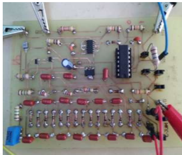
Figure 6: High voltage power supply PCB for GM tube
