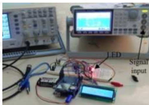
Figure 3: Setup, measurement and testing Arduino Uno output
