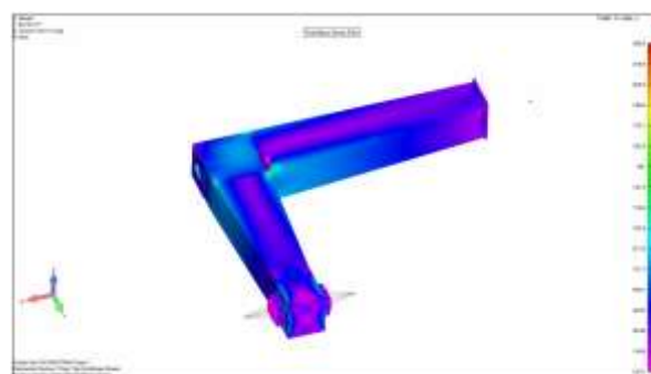
Figure 11: Stress plot of side arm
