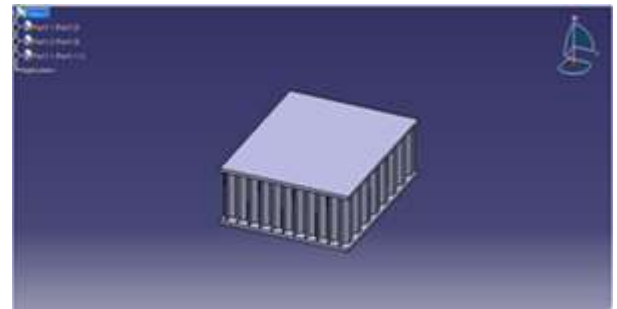
Figure 4.10: Sandwich plate structure in CATIA
