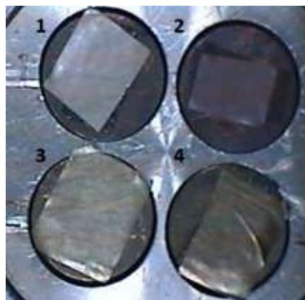
Figure 1: After coating sample images - 1) One minute coating time; 2) Three minute coating time; 3) Five minute coating time; 4) Eight minute coating time
