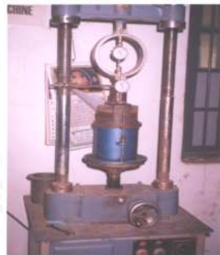
Figure 4: California Bearing Ratio Test Apparatus
