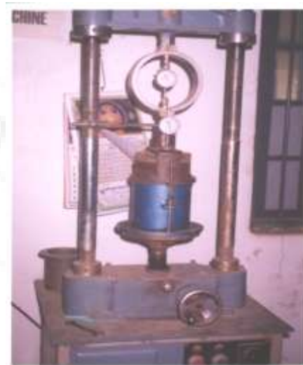
Figure 4: California Bearing Ratio Test Apparatus
