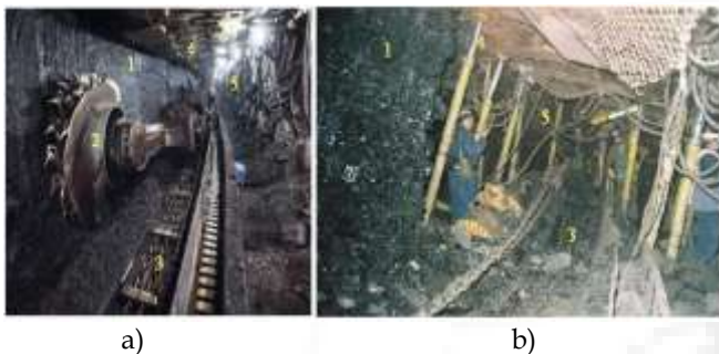
Figure 8: Methods of exploiting coal with combine (a) or drilling-perforation (b)
