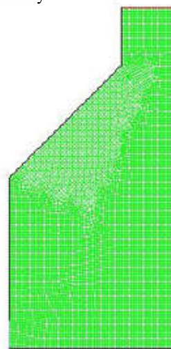
Figure 1: Schematic of two-dimensional solution domain for CFD analysis.
