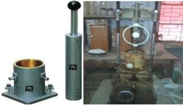
Figure 3: Standard Proctor Test & CBR Apparatus
