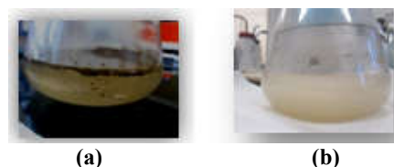
Figure 2: Visual biodegradation of UEO by bacterial consortium compared to the control without bacteria (RT).
