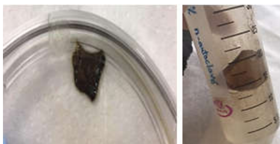
Figure 3: Different samples of the extracellular biopolymer produced by the bacteria consortium grown in 1% UEO.
