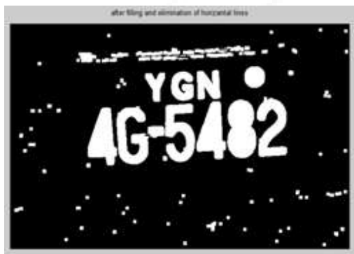
Figure 3.2 (d): filling and elimination of horizontal lines
