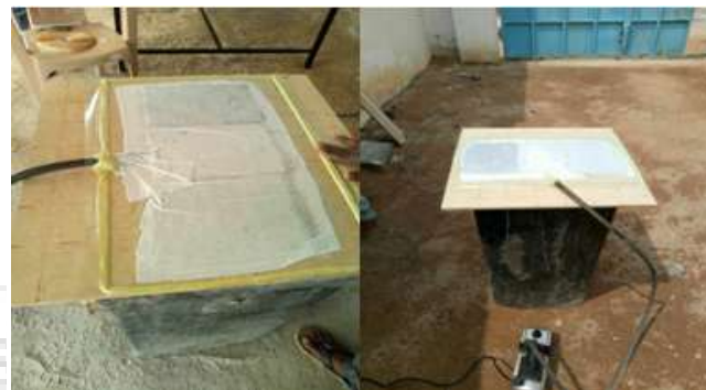
Figure 3.1.1: Vacuum bagging of composite
