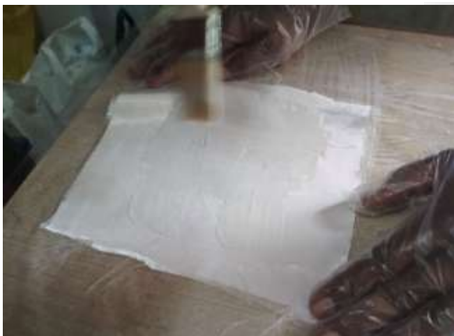
Figure 3.1: Fabrication by hand lay-up technique (compression)
