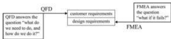
Figure 3 : Integration between QFD and FMEA
