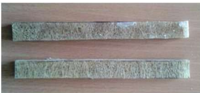
Figure 3.2 (a): Flexural test samples
