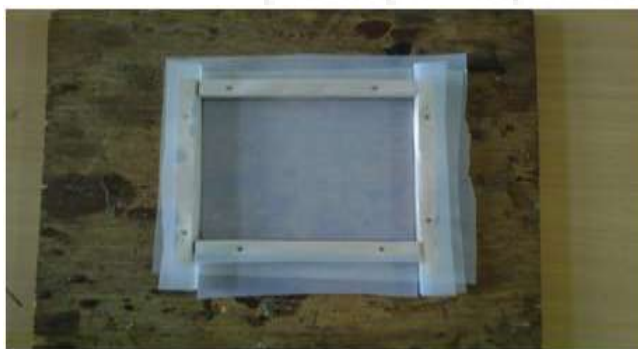
Figure 3.1: Mould used for fabrication of the composite
