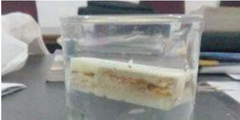
Figure 4.4.1: Water Absorption Test
