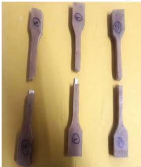
Figure 3.2: Specimen After Fracture
