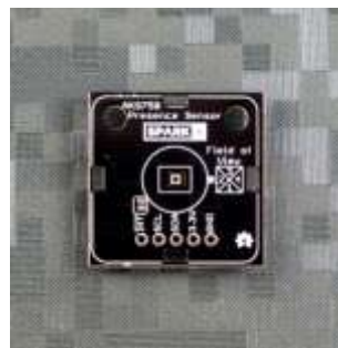
Figure 3: Human Presence sensor AK9750
