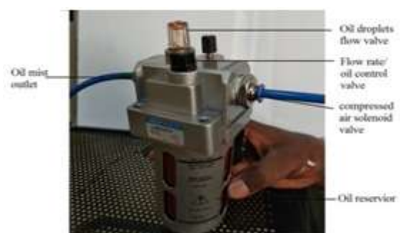
Figure 1: Photographic view of MQL setup
