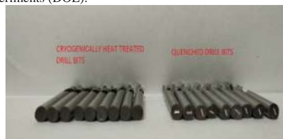
Figure 1: Cryogenically treated and normal heat treated (quenched) drill bits
