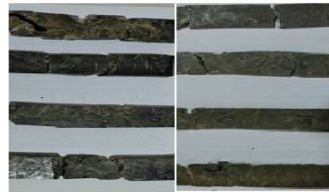
Figure 5: specimen after impact test
