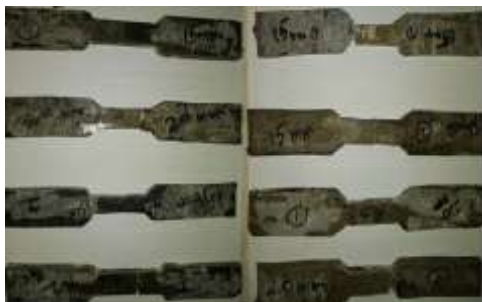
Figure 3: Specimen after tensile test
