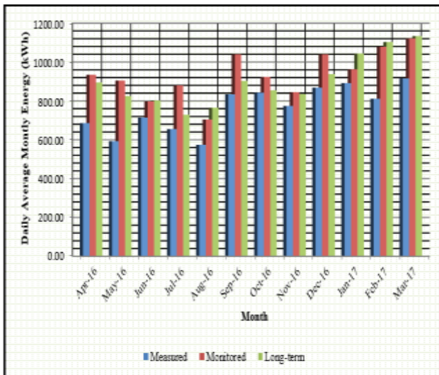
Figure 4: Comparison of Daily Average Monthly Energy based on long-term irradiance, measured irradiance and meter energy supplied to the facility
