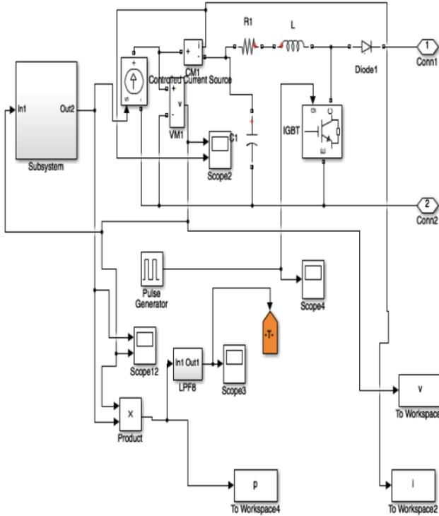
**Figure 6:** Simulation model of PV subsystem without MPPT
