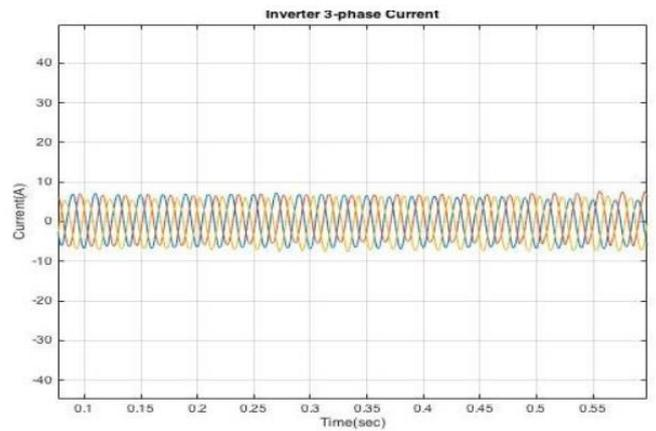
**Figure 14:** Simulated waveform of inverter three-phase current to the load without MPPT
