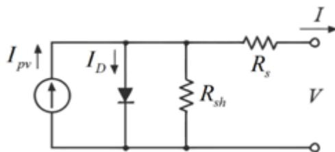
**Figure 1:** Equivalent circuit of a PV cell.
