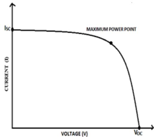
**Figure 2:** V - I characteristic of a solar cell
