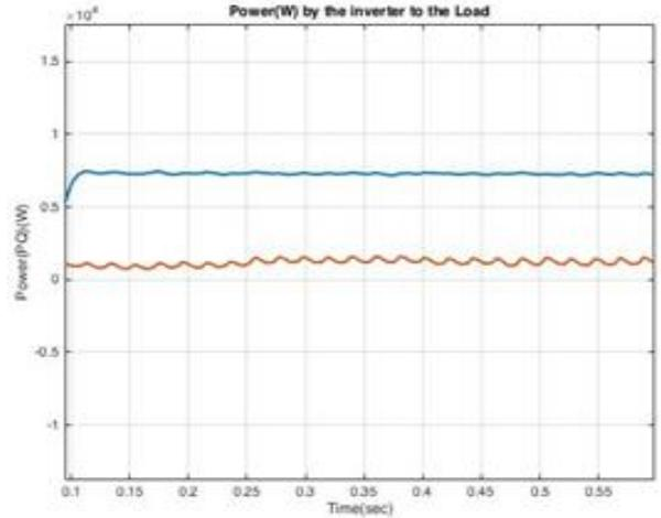
**Figure 8:** Simulation waveform of power from Inverter to the load with MPPT
