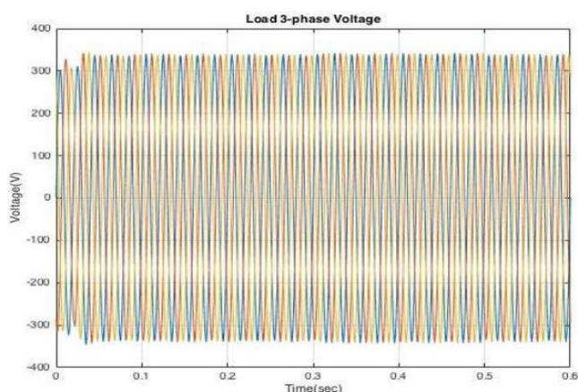
**Figure 18:** Simulated waveform of three-phase load voltage without MPPT
