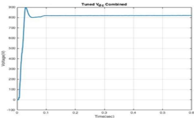
**Figure 7:** Simulated tuned Vdc output waveform with MPPT
