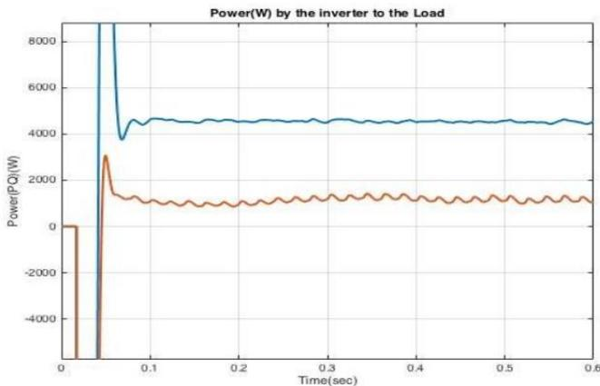
**Figure 13:** Simulation waveform of power from inverter to the load without MPPT
