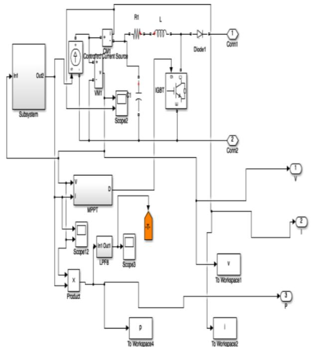
**Figure 5:** Simulation model of PV subsystem with MPPT
