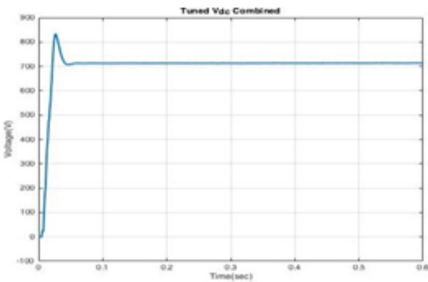
**Figure 12:** Simulated tuned Vdc output waveform without MPPT
