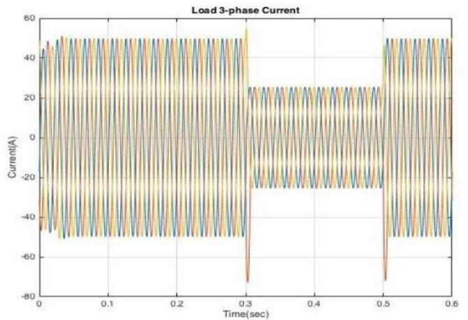
**Figure 15:** Simulated waveform of three-phase load current with MPPT
