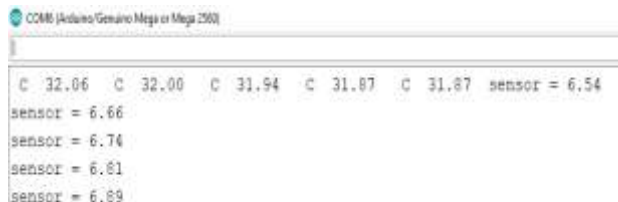
Figure 13: Temperature and pH data readings on Water sample 2
