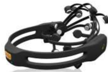
Figure 3: The Emotive Epoc+ Device
