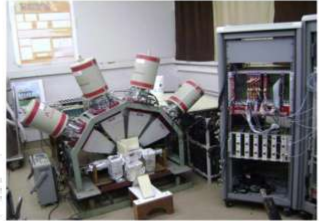
Figure 2.2.1: Clover + LaBr 3 experimental set up at CIRUS laboratory, BARC.
