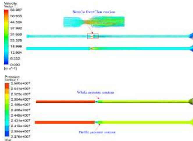
**Figure 4:** The whole velocity vector diagram and the pressure contour When  $Q=10L/s$
