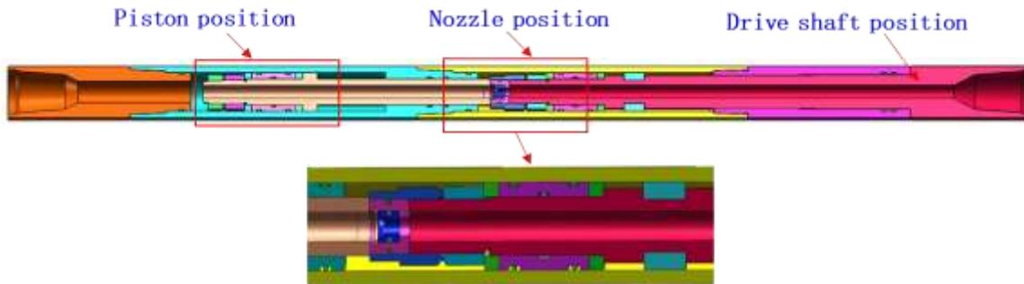
**Figure 1:** The whole and partial enlarged drawing of hydraulic thruster
