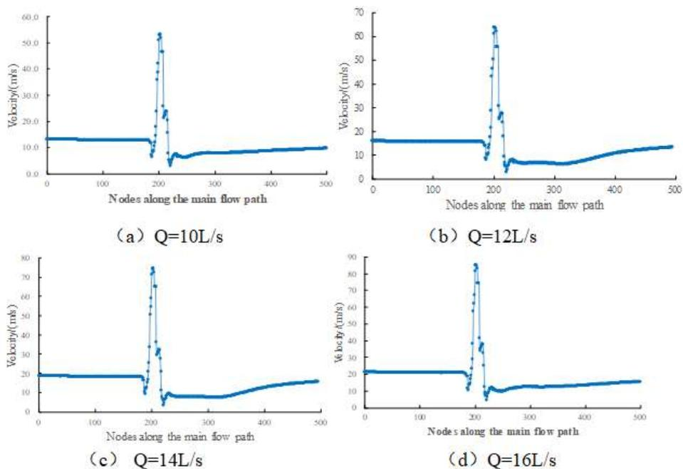
**Figure 8:** Fluid velocity curve on the main path under different flow rates
