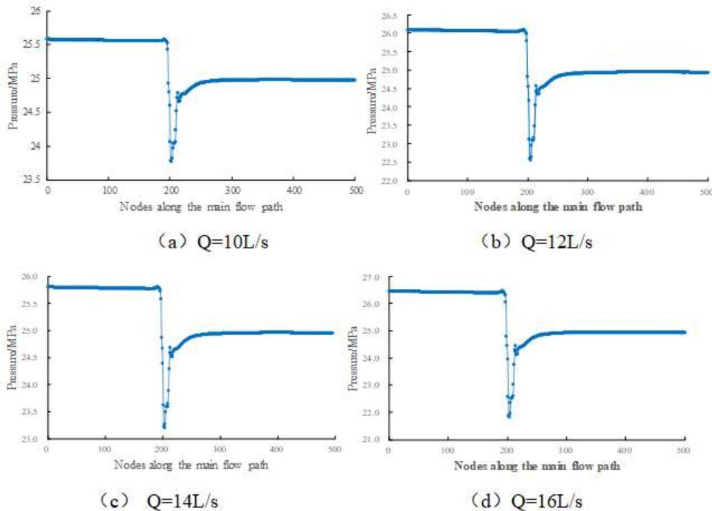
**Figure 9:** Fluid pressure curve on the main path under different flow rates
