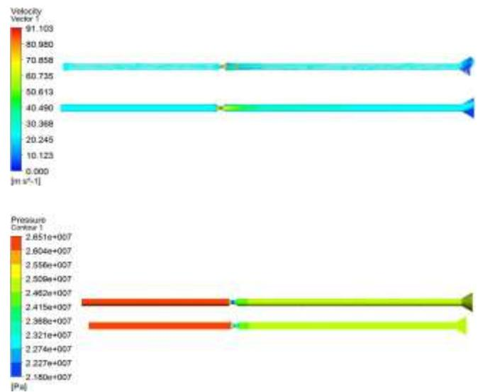
**Figure 7:** The whole velocity vector diagram and the pressure contour When  $Q=16\text{L/s}$
