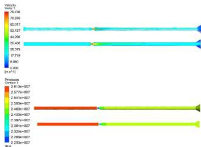
**Figure 6:** The whole velocity vector diagram and the pressure contour When  $Q=14L/s$
