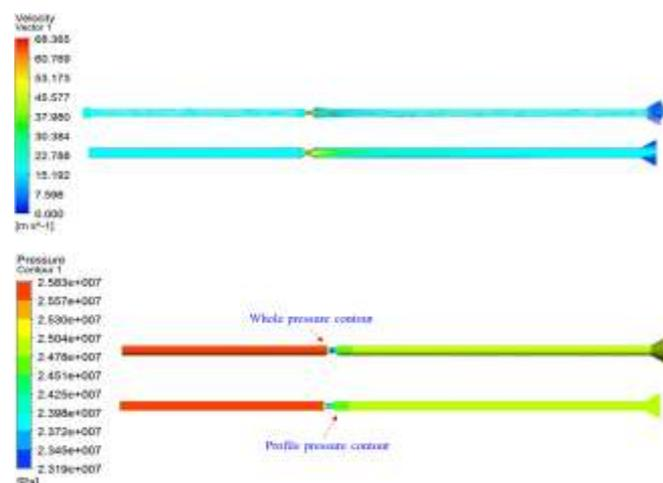
**Figure 5:** The whole velocity vector diagram and the pressure contour When  $Q=12L/s$
