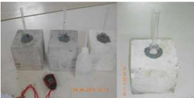
Figure 18: Measurement of water absorption
