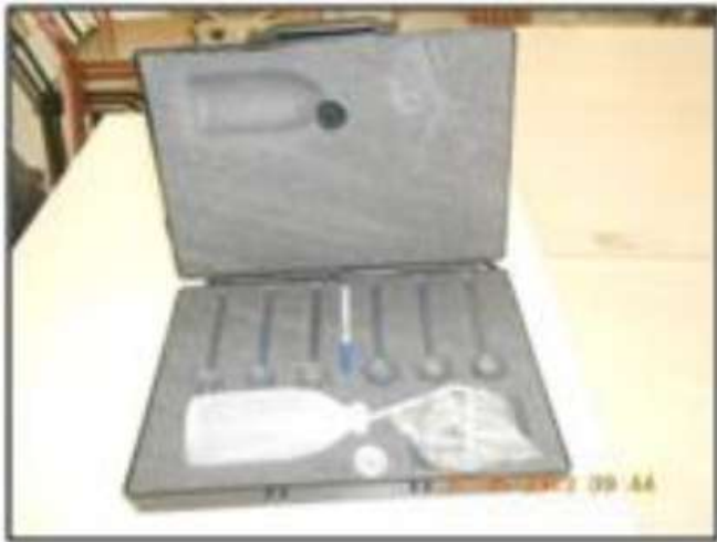
Figure 16: KARSTEN permeability test device
