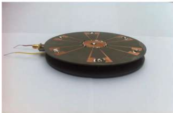
Figure 3: A photo of fabricated omni-directional antenna
