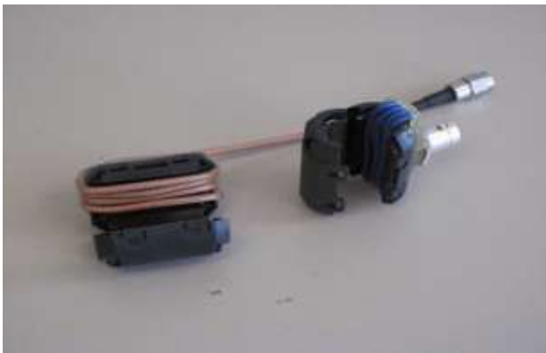
Figure 3: Lab-made current probes
