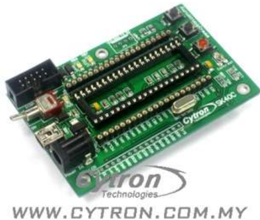
Figure 5: Enhanced 40 pins PIC Start-Up Kit
