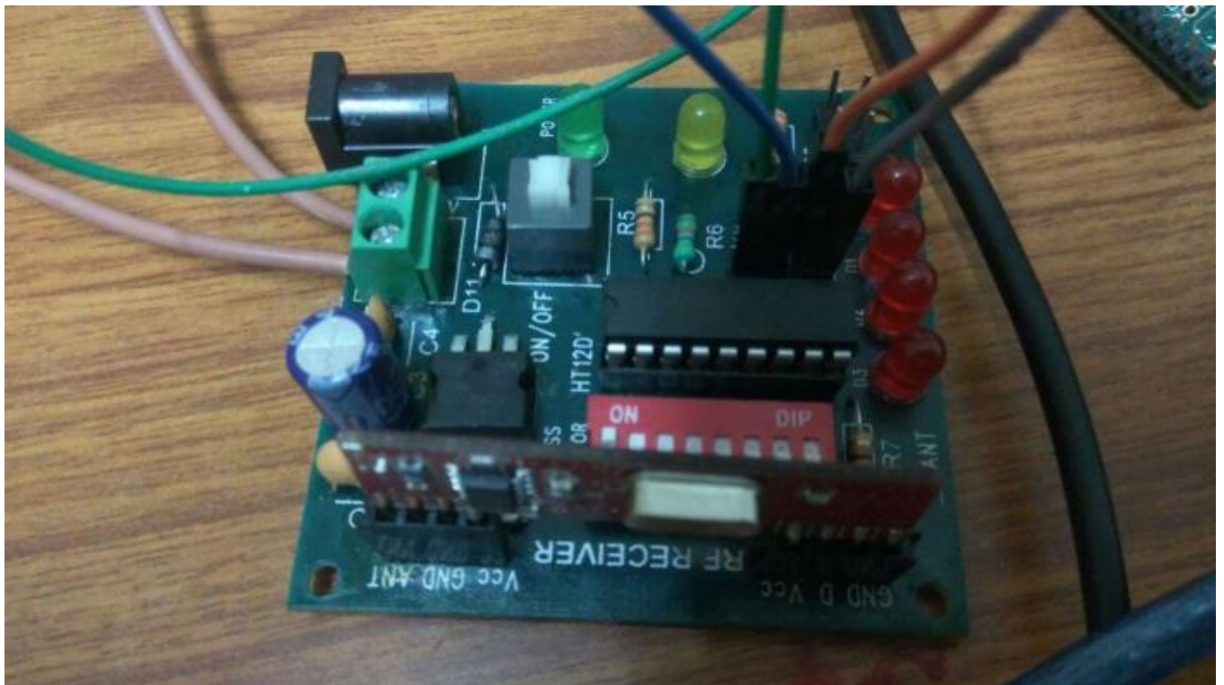
Figure 10: RF Receiver module with decoder
