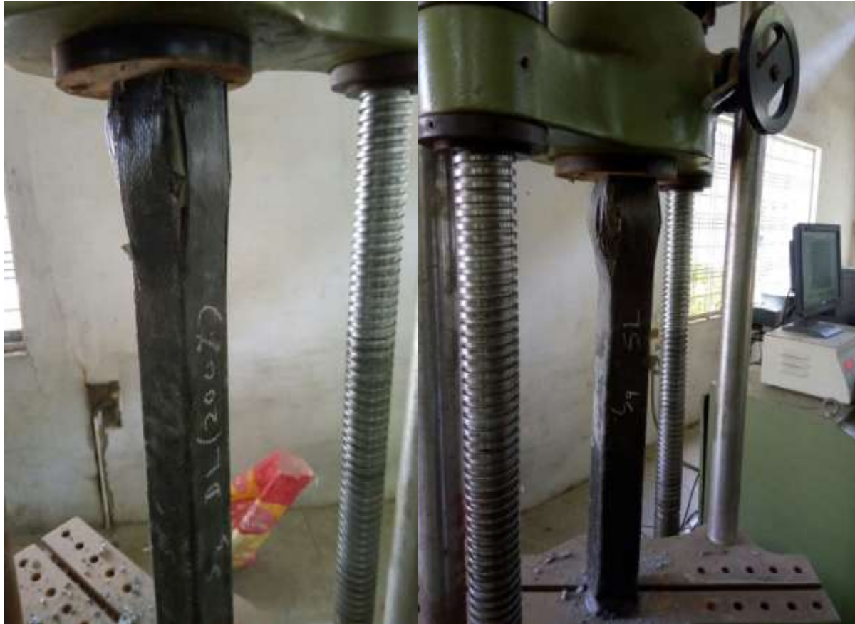
Failure of long column specimens at the ends
