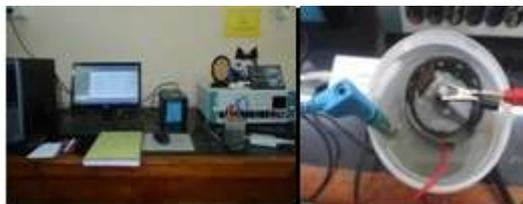
**Figure 4:** Tafel extrapolation test setup
