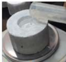
Figure 2.1: Core filled with water Figure 2.2: Refilling the core
