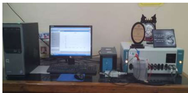
Figure 3.1: Tafel Extrapolation Test setup
