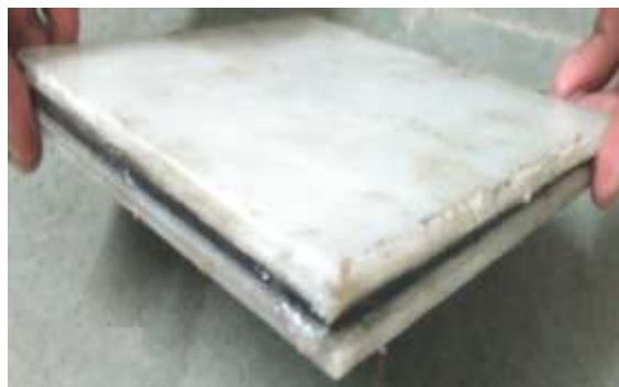
Figure 3: Interply Hybrid Composite Specimen B
