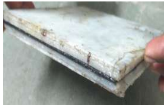
Figure 2: Interply Hybrid Composite Specimen A
