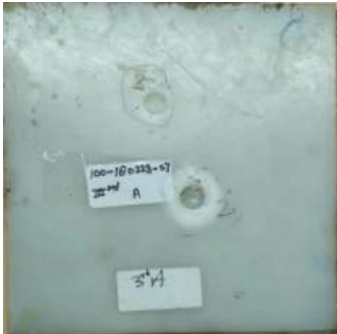
Figure 3: A after Low Velocity Impact Test
