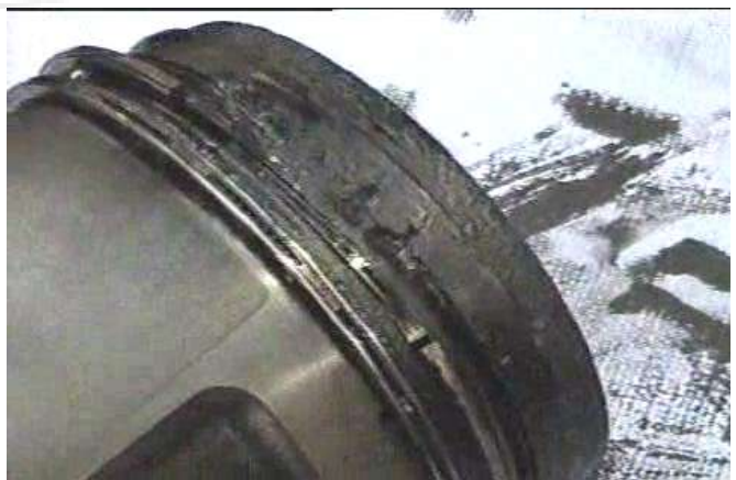
Carbon deposits on the piston above the piston rings – the result of incorrect combustion
