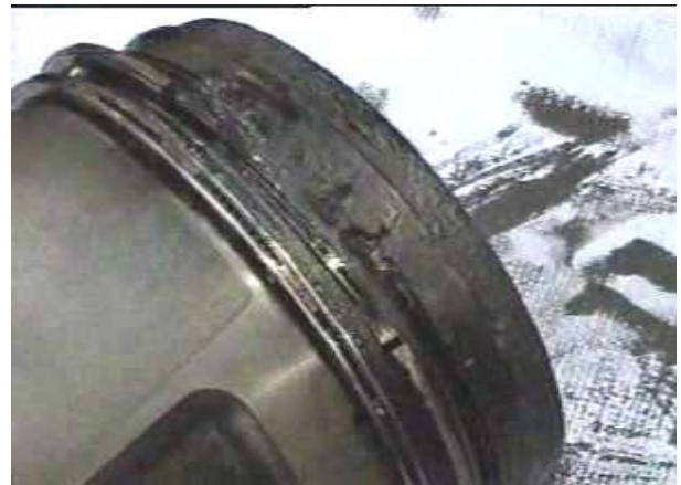
Detailed view of 2 nd cylinder piston immediately after dismantling
