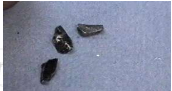
Fragments of the 2 nd cylinder piston found in the engine oil bath after dismantling
