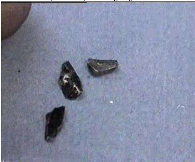
The fragments of the 2 nd cylinder piston found in an oil bath – traces of blows on the moving parts of an engine
