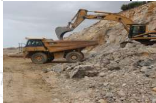
Figure 3: Loading equipment and truckloads on a career scale [Source: Photo from authors, Fushë Krujë].
