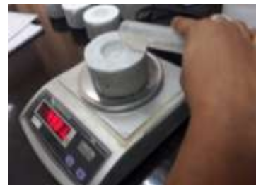
Figure 3.1: Measuring of weight of dry and filed specimen
