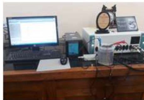
Figure 4.2: Experimental setup of TAFEL Extrapolation
