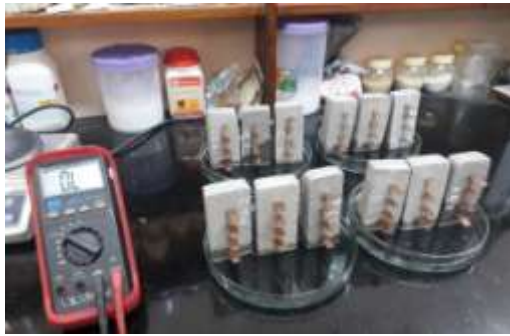
Figure 2.1: Electrical resistance test for bar specimens
