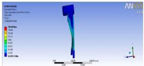
**Figure 17:** Maximum von-mises stresses at 500N
