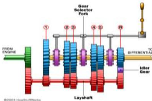
**Figure 3:** 5 speed manual transmission
