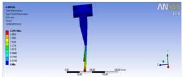
**Figure 15:** Total deformation at 1500N
