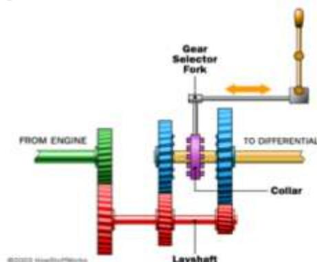
Figure 1: Simple 2 speed transmission
