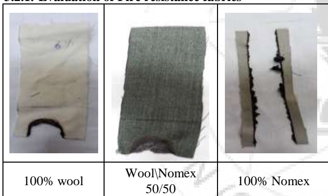
Figure 8: The digital photos for the tested sample after vertical burning tests.
