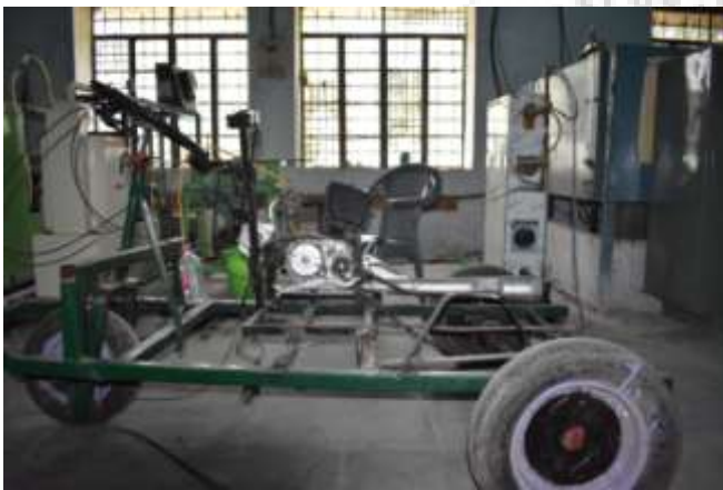
Figure 5: Side view after engine mounting
