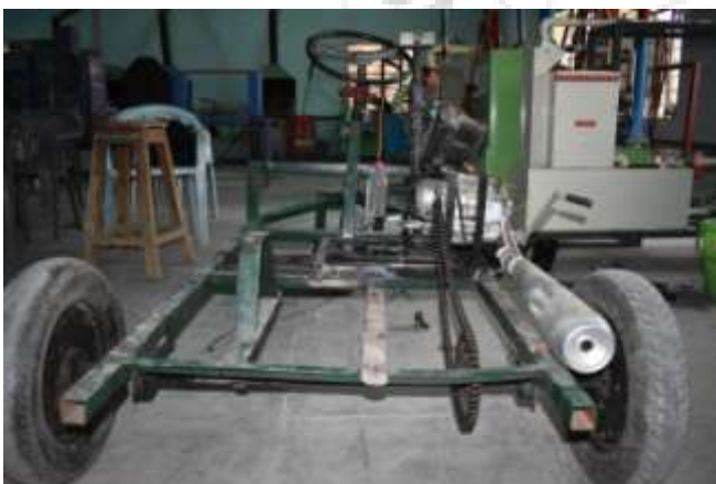
Figure 6: rear view after engine mounting
