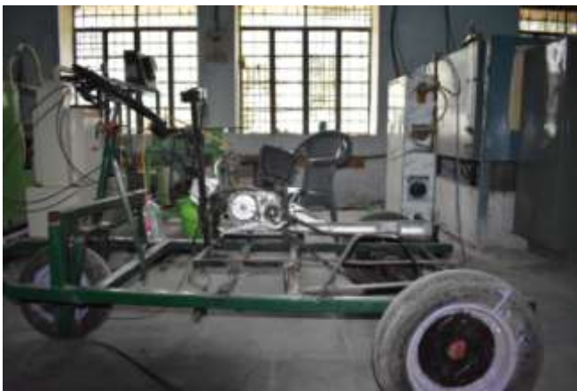
Figure 5: Side view after engine mounting
