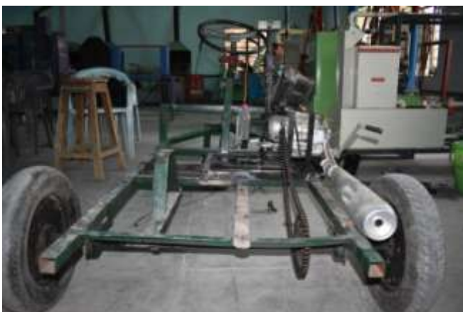
Figure 6: rear view after engine mounting
