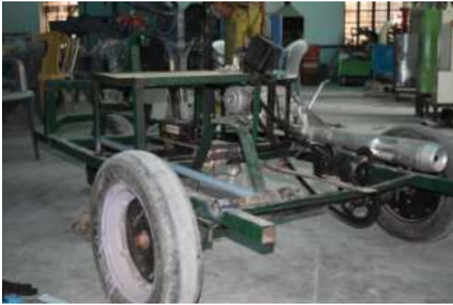
Figure 4: Rear wheel installation
