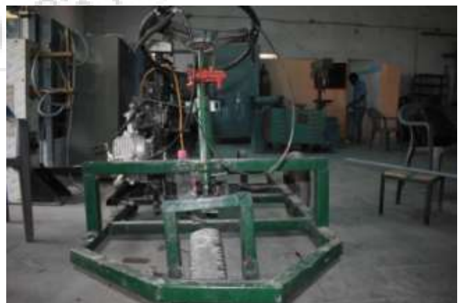
Figure 3: Front wheel and steering wheel installation
