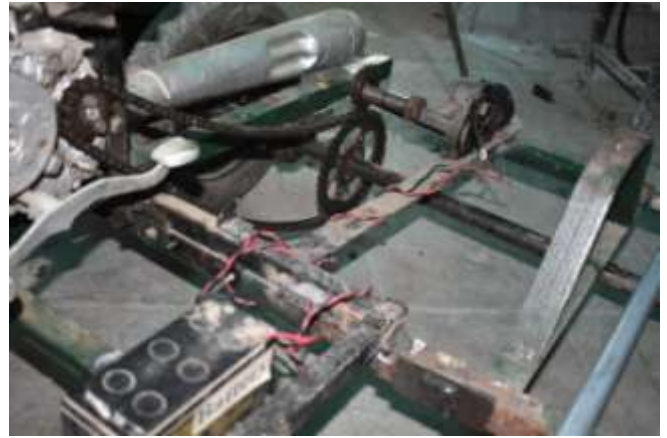
Figure 7: mounting of dc motor and battery
