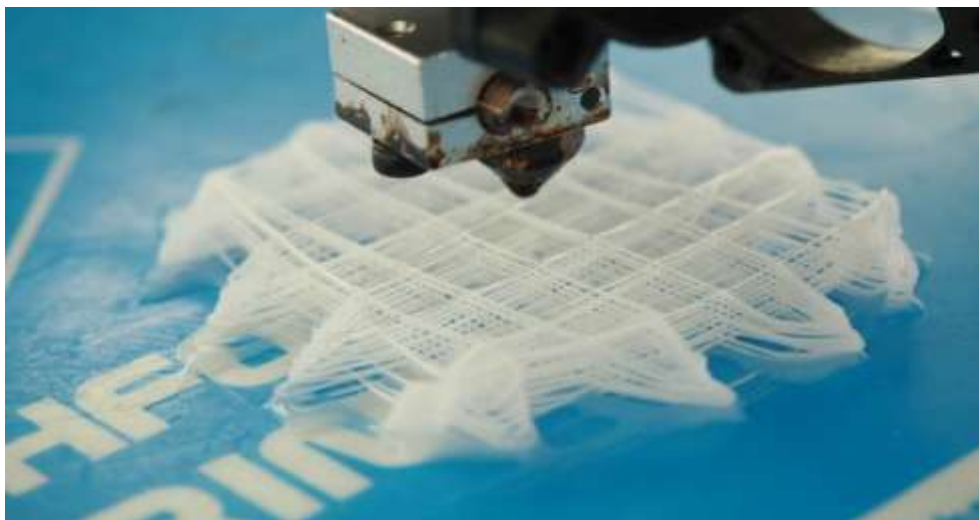
3D Printing of a breast tissue scaffold
