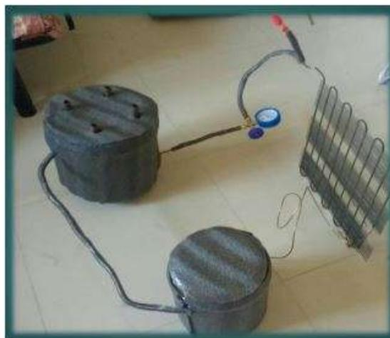
Figure 9: Developed Adsorption Refrigeration System
