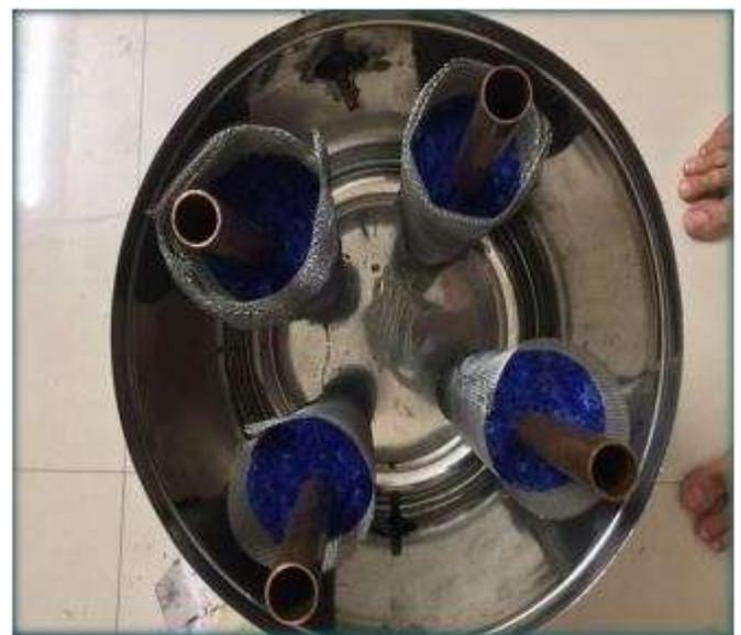
**Figure 4: Fabricated Adsorber Bed**
