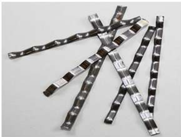
Figure 2: crimped steel fiber
