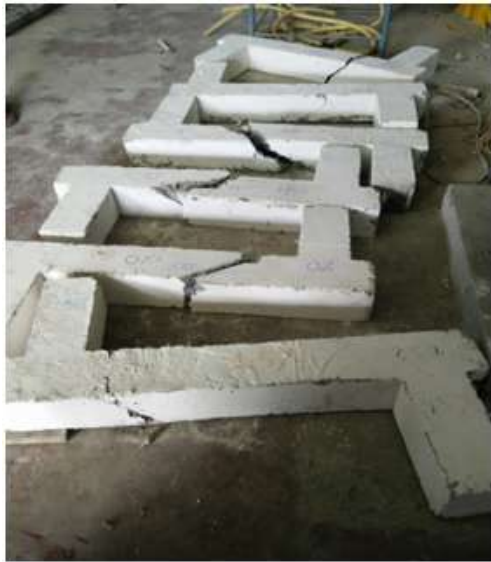
Figure 6: Failure of beams
