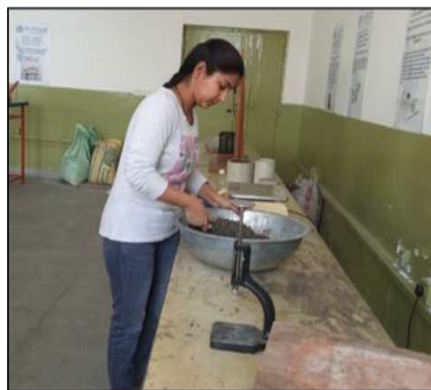
Figure 3: Mixing of concrete material for slump test
