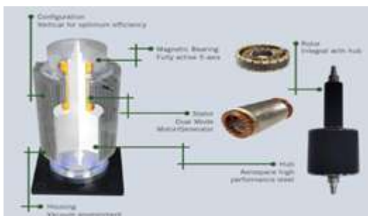
Figure 3: Internal construction of flywheel assembly includes the housing, stator, rotor, hub, and magnetic bearings
