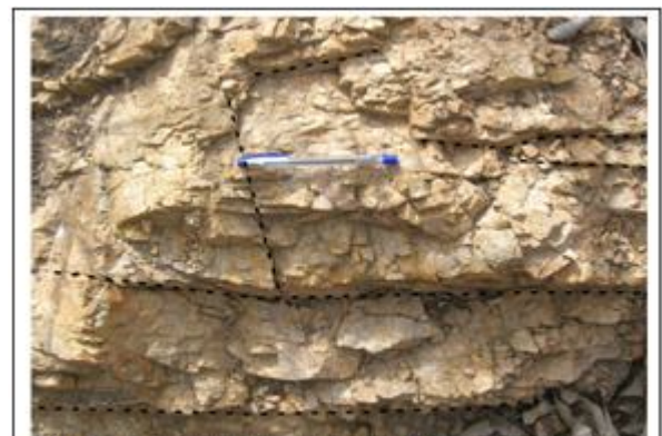
Photo 2: Cataclasis area, in the pan-African quartzitic base, linked to Kandi's N10° to N30° fault. The outcrop width of the noncohesive cataclasite varies from 1 to 2 m. (Tondika, South Gaya)
