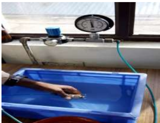
Figure 2.2.1: water immersion test
