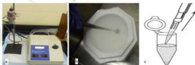
Figure 3: a) Homogenization of fish tissue specimens b) Shocking of tissue specimens in liquid nitrogen c) Collecting of supernatant
