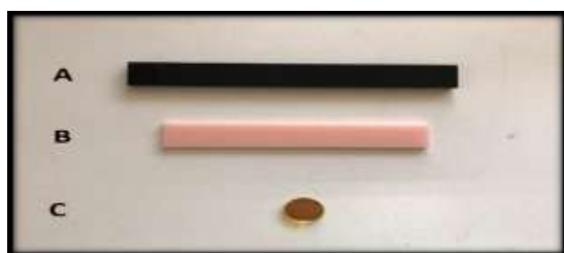
Figure 1: plastic models used in the study; A for Impact strength, B for transverse strength specimen and C for antibacterial activity test specimens
