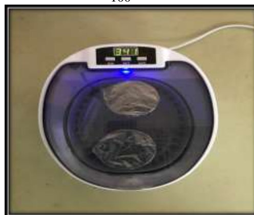
Figure 4: disinfectant treatment of acrylic specimens under ultrasonic waves
