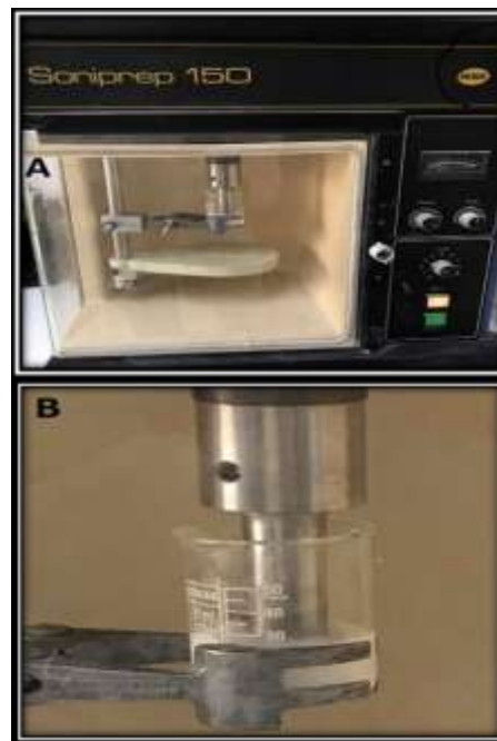
Figure 2: A, B nanofillers' dispersion within the monomer by Ultrasonic disintegrator
